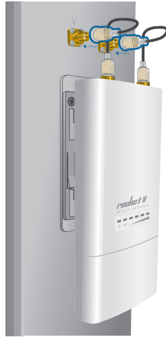
Connecting to a Sector Antenna
