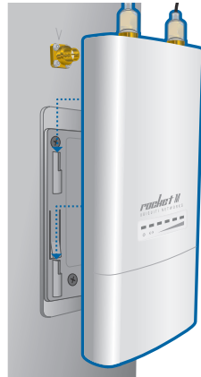
Mounting on a Sector Antenna
