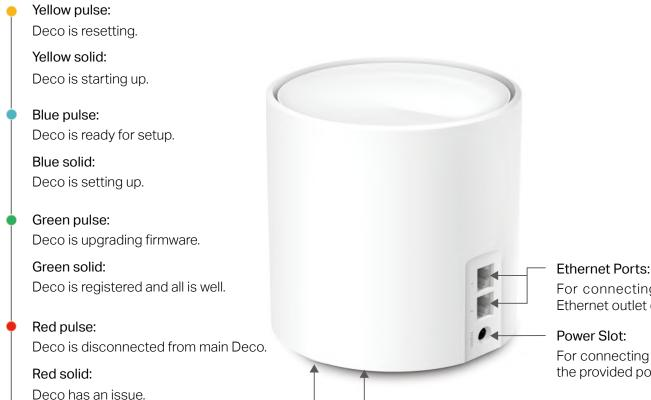
For connecting Deco to your modem, the Ethernet outlet or other internet devices.
