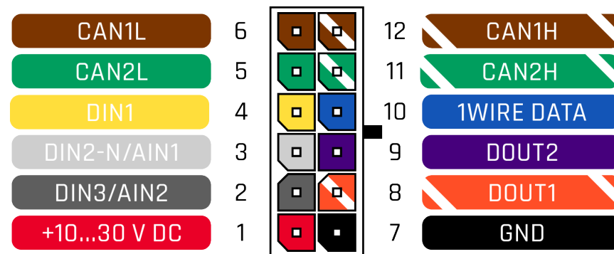
Figure 2 FMB140 2x6 socket pinout
