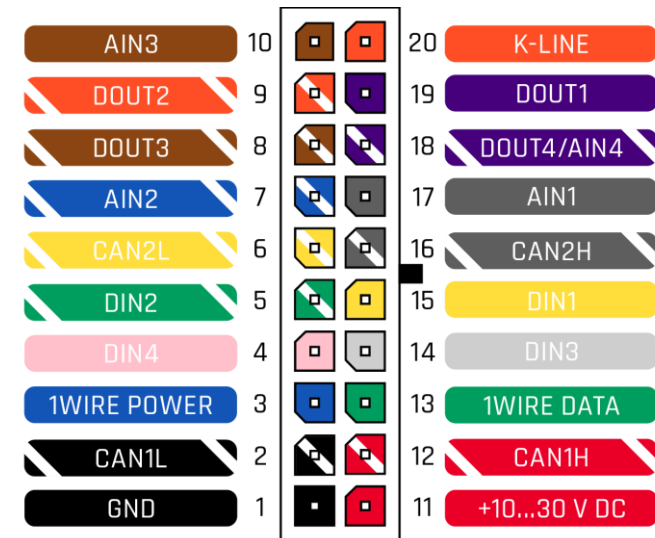
Figure 2 FMC640 pinout
