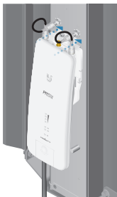
Connecting to a Sector Antenna
