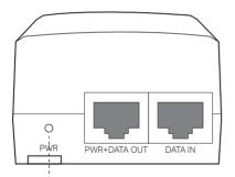
On: Supplying power normally Off: No power supply
