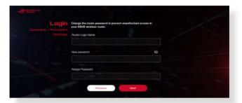
**NOTE:** The wireless router's login username and password is different from the 2.4GHz/5GHz/6GHz network name (SSID) and security key. The wireless router's login username and password allows you to log into your wireless router's Web GUI to configure your wireless router's settings. The 2.4GHz/5GHz/6GHz network name (SSID) and security key allows Wi-Fi devices to log in and connect to your 2.4GHz/5GHz/6GHz network.
