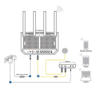
Connect to the network name (SSID) shown on the product label on the back side of the router. For better network security, change to a unique SSID and assign a password.
