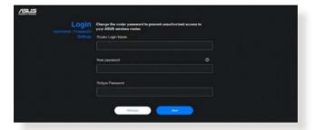
**NOTE:** The wireless router's login username and password is different from the 2.4GHz/5GHz/6GHz network name (SSID) and security key. The wireless router's login username and password allows you to log into your wireless router's Web GUI to configure your wireless router's settings. The 2.4GHz/5GHz/6GHz network name (SSID) and security key allows Wi-Fi devices to log in and connect to your 2.4GHz/5GHz/6GHz network.
